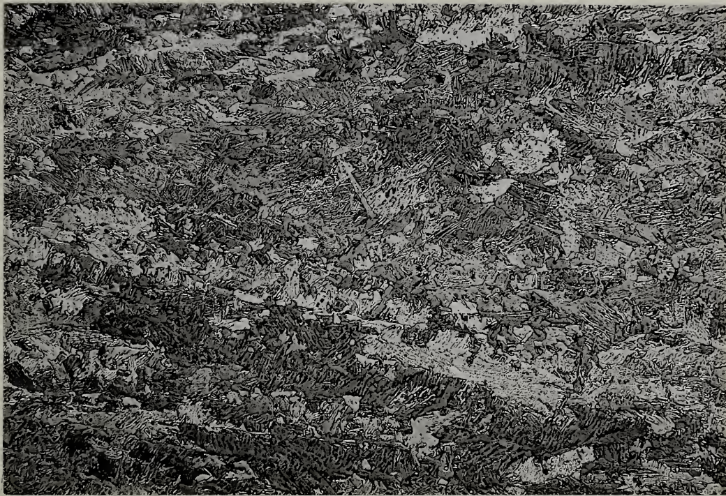
Figure 10. Microstructure of weld material. 1% Nital etch. X 100
